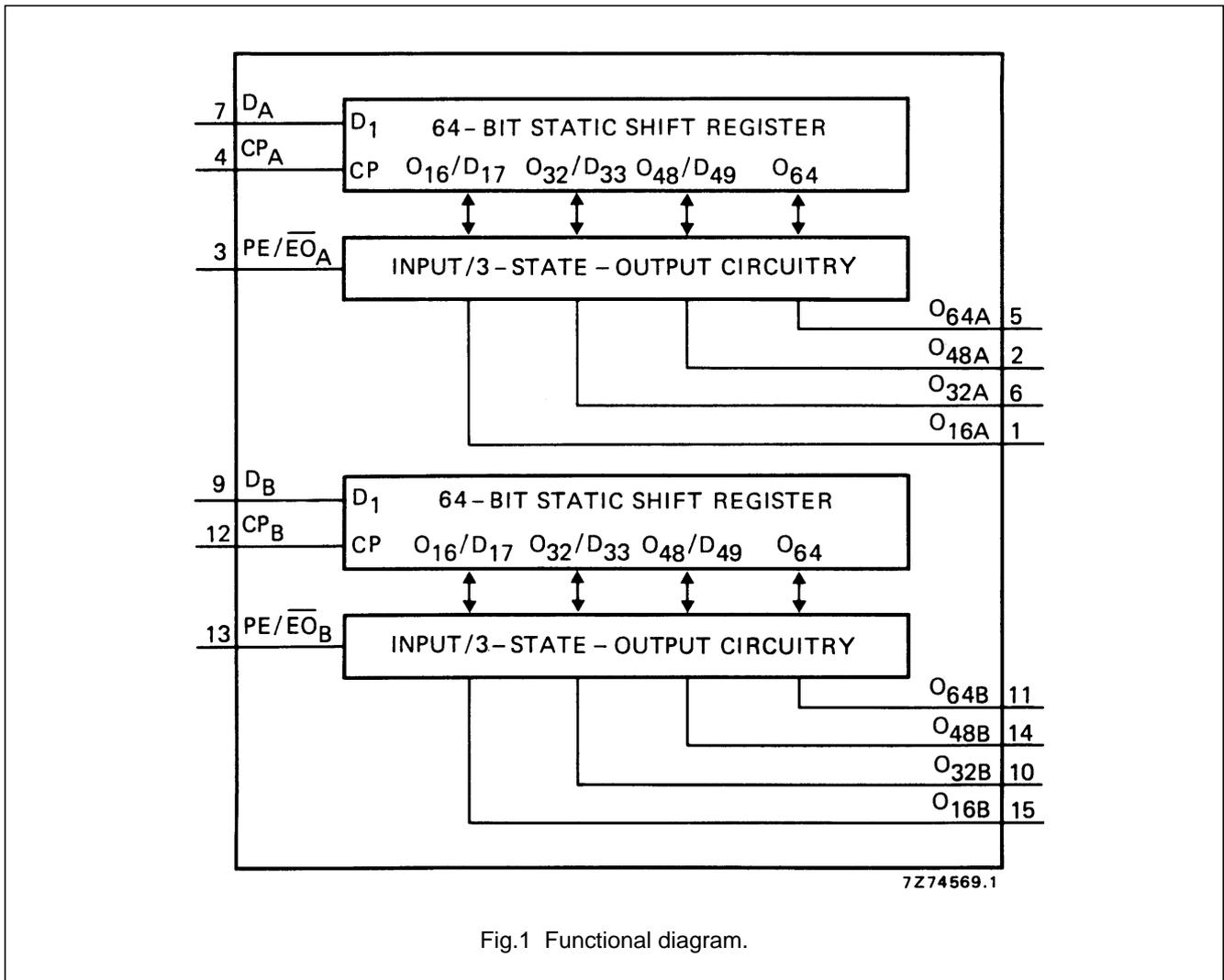
Fig.1 Functional diagram.
