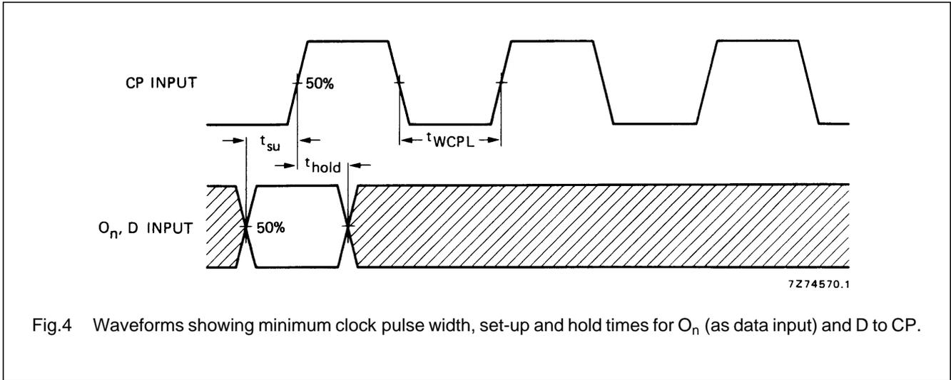
Fig.4 Waveforms showing minimum clock pulse width, set-up and hold times for O<sub>n</sub> (as data input) and D to CP.
