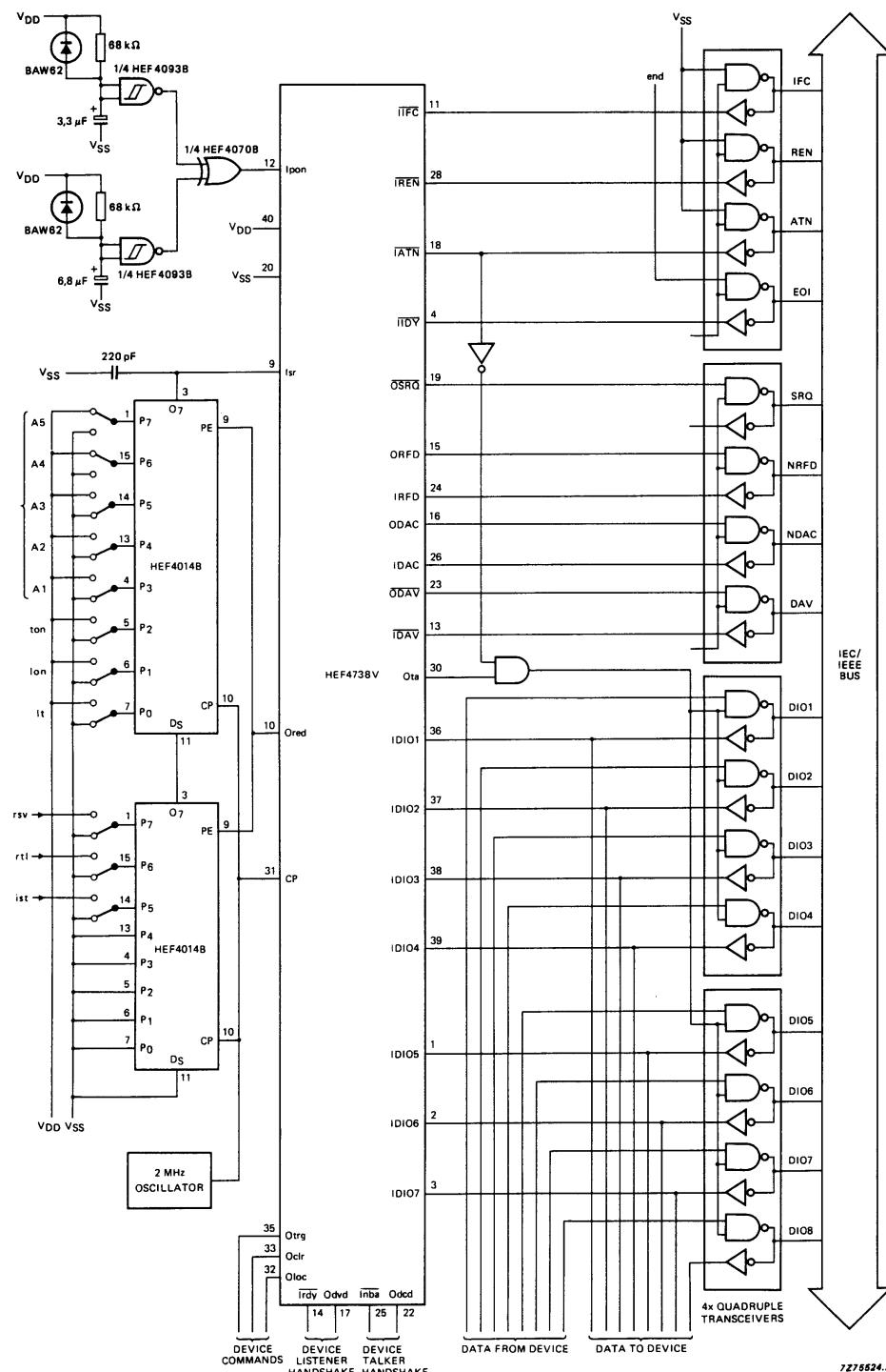
Fig.6 Basic listener and talker. Serial and parallel poll are not implemented.
