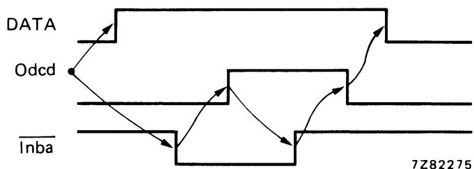
Fig.4 Waveforms showing data exchange in talker function.
