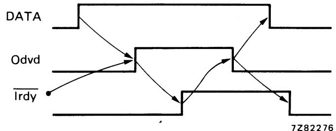
Fig.5 Waveforms showing data exchange in listener function.
