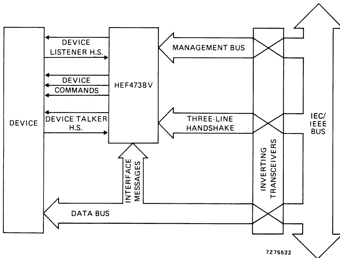
Fig.1 Basic IEC/IEEE bus interface using the HEF4738V.
