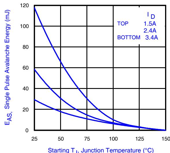
**Fig 14.** Maximum Avalanche Energy vs. Drain Current
