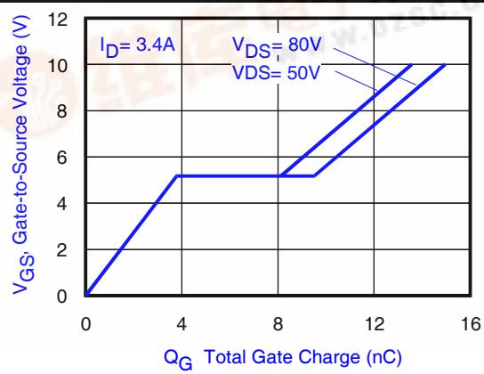
Fig 2. Typical Total Gate Charge vs. Gate-to-Source Voltage
