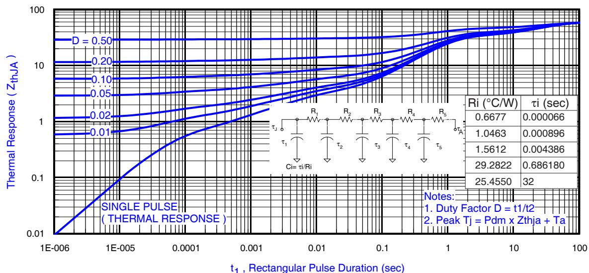
Fig 3. Maximum Effective Transient Thermal Impedance, Junction-to-Ambient ①
