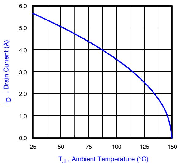
**Fig 12.** Maximum Drain Current vs. Ambient Temperature
