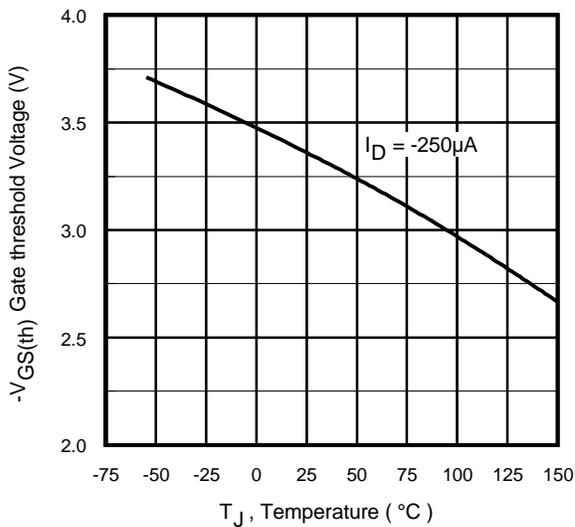
**Fig 33.** Typical Threshold Voltage Vs. Junction Temperature
