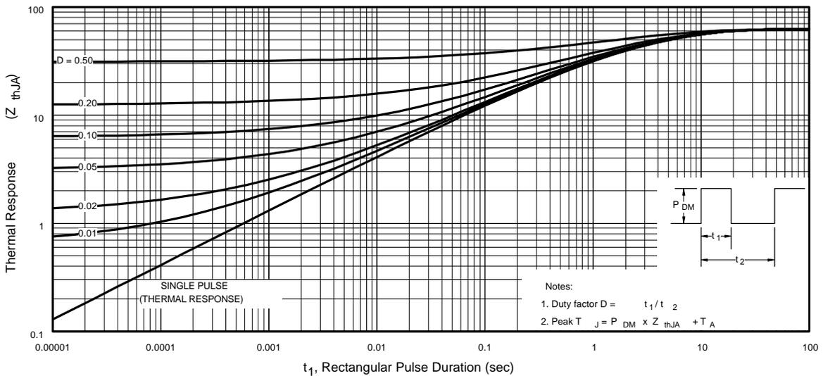
**Fig 11.** Typical Effective Transient Thermal Impedance, Junction-to-Ambient
