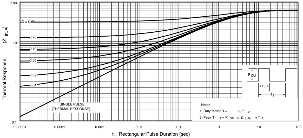
**Fig 30.** Typical Effective Transient Thermal Impedance, Junction-to-Ambient
