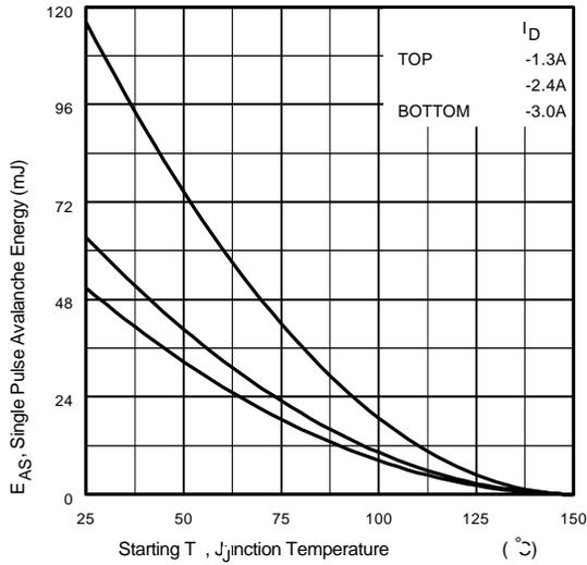
Fig 35a. Maximum Avalanche Energy Vs. Drain Current
