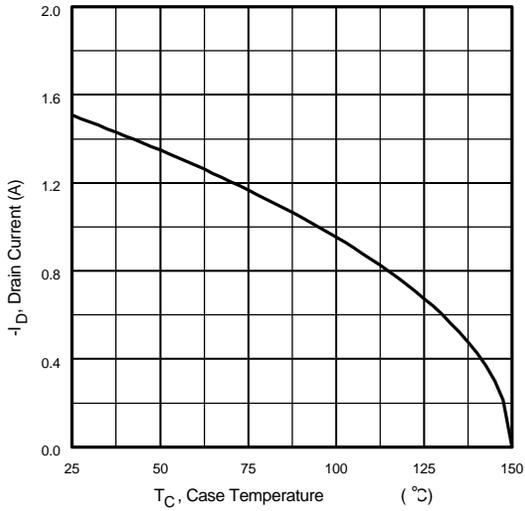
**Fig 29.** Maximum Drain Current Vs. Case Temperature
