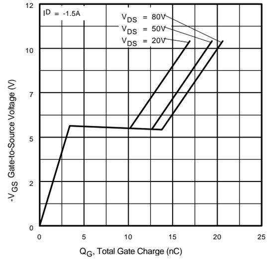
**Fig 26.** Typical Gate Charge Vs. Gate-to-Source Voltage
