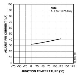
Figure 7. Adjust Pin Current vs. Temperature
