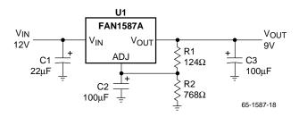
Figure 15. Application Circuit (FAN1587A)
