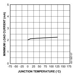
Figure 6. Minimum Load Current vs. Temperature
