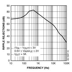
Figure 9. Ripple Rejection vs. Frequency
