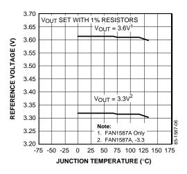
Figure 5. Output Voltage vs. Temperature
