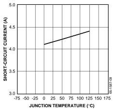
Figure 8. Short-Circuit Current vs. Temperature
