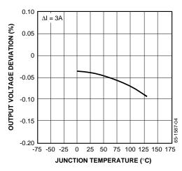
Figure 3. Load Regulation vs. Temperature
