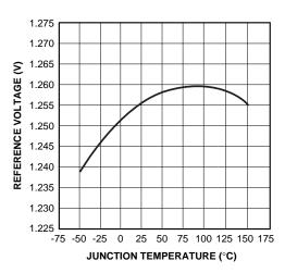
Figure 4. Reference Voltage vs. Temperature
