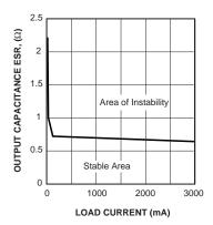
Figure 11. Stability Region V<sub>IN</sub>/V<sub>OUT</sub> = 5V/1.5V
