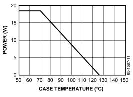
Figure 10. Maximum Power Dissipation
