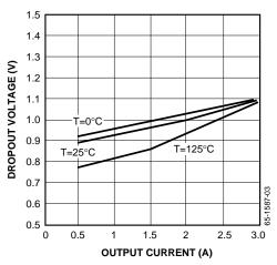
Figure 2. Dropout Voltage vs. Output Current
