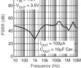
Power Supply **Rejection Ratio** I<sub>OUT</sub> = 150mA COUT = 10µF Cer
