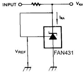
Figure 1. Test Circuit for  $V_{KA} = V_{REF}$
