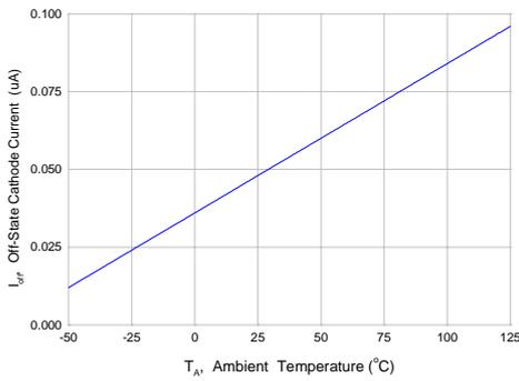
Figure 6. OFF-State Cathode Current vs. Ambient Temperature
