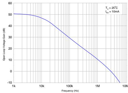
Figure 8. Small Signal Voltage Amplification vs. Frequency
