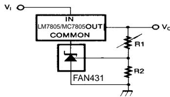
Figure 14. Output Control for Three-Terminal Fixed Regulator
