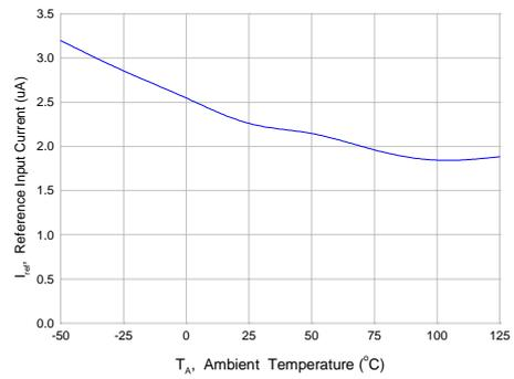
Figure 7. Reference Input Current vs. Ambient Temperature
