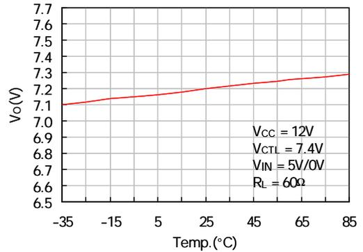
Figure 4. Temperature vs V<sub>O</sub>
