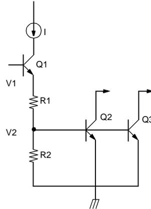
When  $T_a = 25^\circ\text{C}$ , Q2 & Q3 are Turned-off and output stage operates normally.
