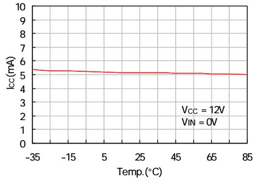
Figure 2. Temperature vs I<sub>CC</sub>
