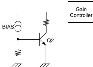
When the chip temperature rises up to about 175°C, the Q2 turns on so that the output driver shuts down. When the chip temperature falls off to about 150°C, then the Q2 turns off so that the driver is to operate normally. TSD has the temperature hysteresis of about 25°C.
