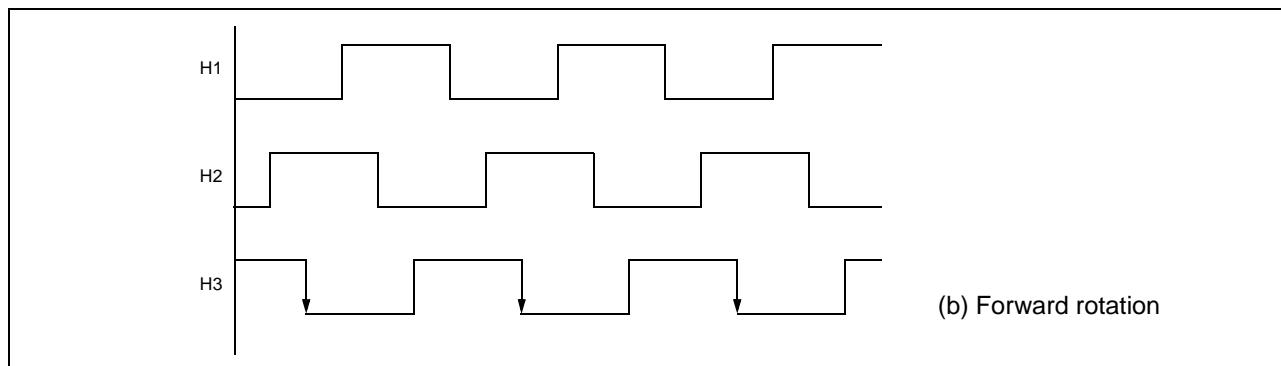
Therefore, the output of the rotational direction detector is Low, when the spindle rotates forward, while HIGH as in the case of the reverse rotation.
