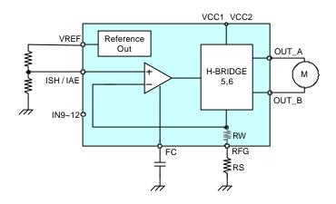
Motor current is determined by ISH/IAE voltage and Rs sensing resistance and calculated by the formula below considering Rw. Generally internal bonding and metal resistance Rw is around  $0.05\Omega$ .
