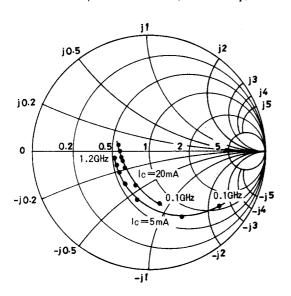
$S12e: V_{CE} = 10V \\ f = 100 MHz, 200 \text{ to } 1200 MHz \text{ (200MHz step)}$
