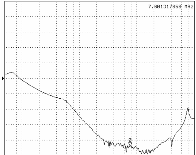
Fig. 3: Common Mode attenuation, 0.05-100 MHz. Source and load resistances are 50 \Omega . Two 0.1 \mu F Y-caps to common line. Vertical scale: 20 dB/div, with zero dB level marked by arrow.
