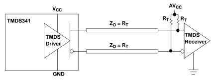
Figure 32. TMDS Driver and Termination Circuit
