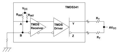
Figure 31. TMDS Input Fail-Safe Recommendation
