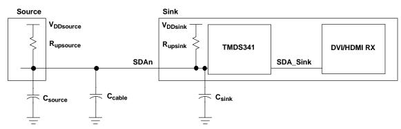
Figure 38. DDC Link From Source to Sink Without External Switch Box
