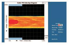
Figure 35. Eye Diagram at Output 10-m 28-AWG Cable vs TP2 Eye Mask
