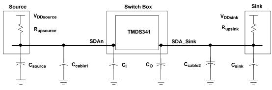
Figure 37. DDC Link from Source to Sink With External Switch Box
