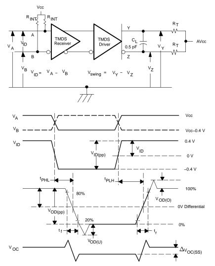
NOTE: All input pulses are supplied by a generator having the following characteristics:  $t_r$  or  $t_f < 100$  ps, 100 MHz from Agilent 81250.  $C_L$  includes instrumentation and fixture capacitance within 0.06 m of the D.U.T. Measurement equipment provides a bandwidth of 20 GHz minimum.
