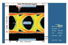
Figure 36. Eye Diagram Recovered by TMDS341 vs TP2 Eye Mask
