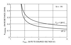
Figure 3. On-Resistance Variation with Temperature.
