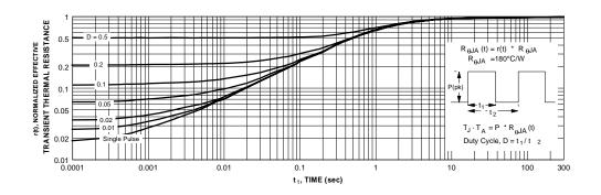
Figure 11. Transient Thermal Response Curve.
