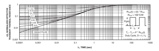
Figure 11. Transient Thermal Response Curve.
