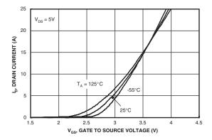
Figure 5. Transfer Characteristics.
