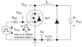
Figure 12. Unclamped Inductive Load Test Circuit
