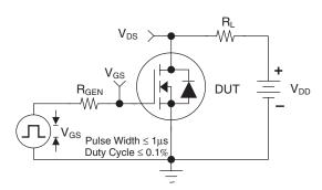
Figure 16. Switching Time Test Circuit
