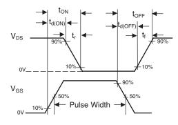
Figure 17. Switching Time Waveforms
