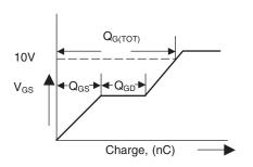
Figure 15. Gate Charge Waveform
