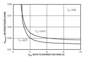
Figure 4. On-Resistance Variation with Gate-to-Source Voltage.
