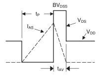
Figure 13. Unclamped Inductive Waveforms
