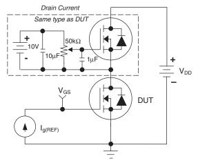
Figure 14. Gate Charge Test Circuit
