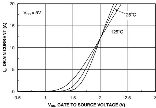
Figure 5. Transfer Characteristics.
