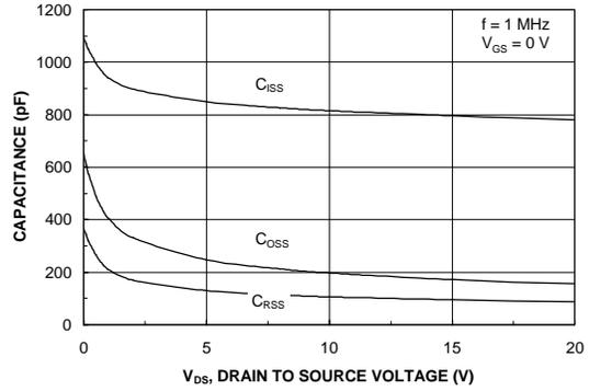
**Figure 8. Capacitance Characteristics.**
