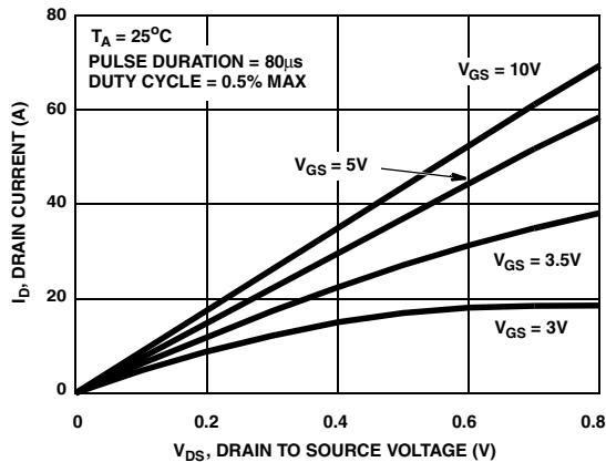
**Figure 7. Saturation Characteristics**
