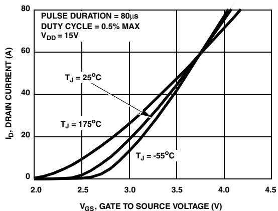
**Figure 6. Transfer Characteristics**
