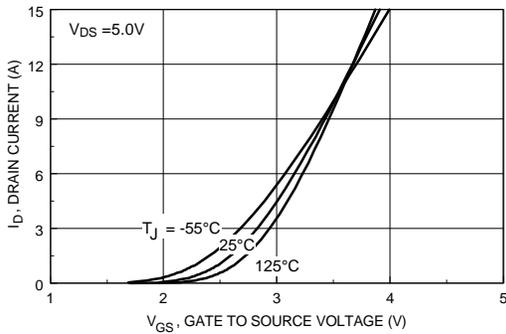
Figure 5. Transfer Characteristics.
