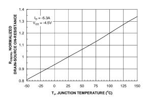
Figure 3. On-Resistance Variation with Temperature.
