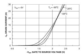
Figure 5. Transfer Characteristics.
