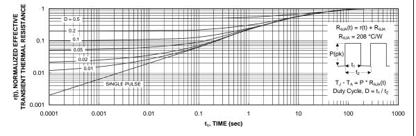
Figure 11. Transient Thermal Response Curve.
