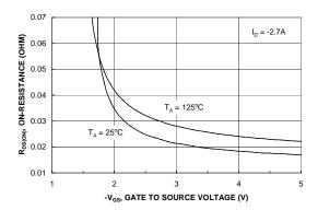
Figure 4. On-Resistance Variation with Gate-to-Source Voltage.
