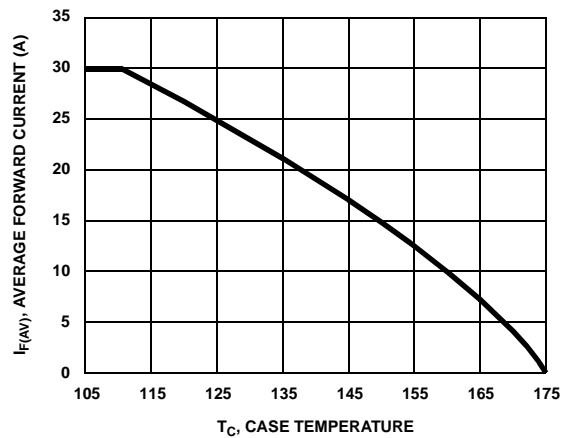
Figure 10. DC Current Derating Curve
