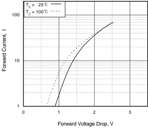
Fig 18. Forward Characteristics
