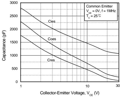
**Fig 7. Capacitance Characteristics**
