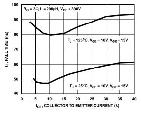
Figure 12. Fall Time vs Collector to Emitter Current
