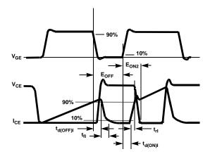
Figure 21. Switching Test Waveforms
