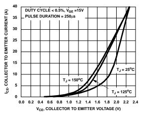
Figure 6. Collector to Emitter On-State Voltage
