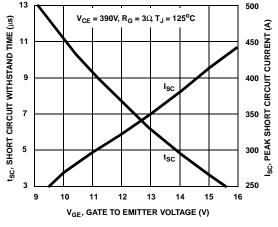
Figure 4. Short Circuit Withstand Time
