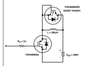
Figure 20. Inductive Switching Test Circuit
