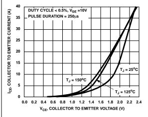
Figure 5. Collector to Emitter On-State Voltage
