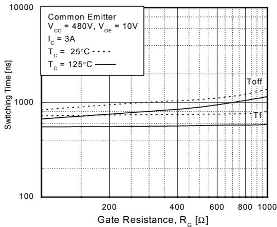
**Figure 10. Switching Loss vs. Gate Resistance**
