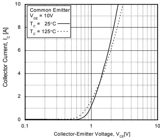
**Figure 4. Transfer Characteristics**
