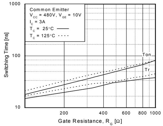
**Figure 9. Turn-Off Characteristics vs. Gate Resistance**
