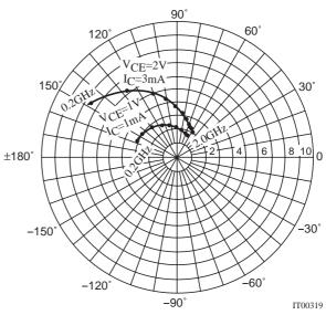
$f{=}200 MHz$  to  $2000 MHz (200 MHz\ Step)$  S22e
