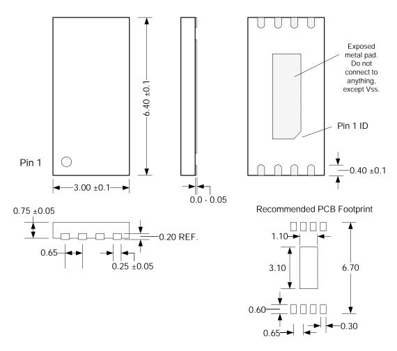
Note: All dimensions in millimeters. This package is footprint compatible with the 8-pin TSSOP.
