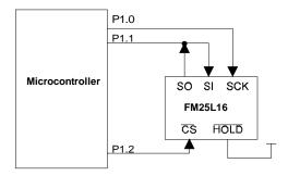
Figure 3. System Configuration without SPI port
