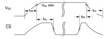
**Data Retention**  $(V_{DD} = 2.7 \text{V to } 3.6 \text{V}, +85^{\circ} \text{ C})$
