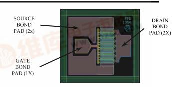
DIE SIZE: 470 x 440 μm DIE THICKNESS: 100 μm BONDING PADS: >85 x 60 μm
