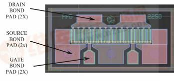
DIE SIZE (μm):: 680 x 470 DIE THICKNESS: 75 μm BONDING PADS (μm): > 85 x 60
