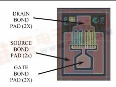
DIE SIZE (µm): 340 x 470 DIE THICKNESS: 75 µm BONDING PADS (µm): >60 x 60
