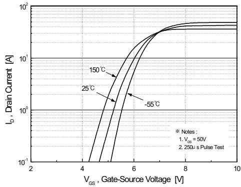
**Figure 2. Transfer Characteristics**
