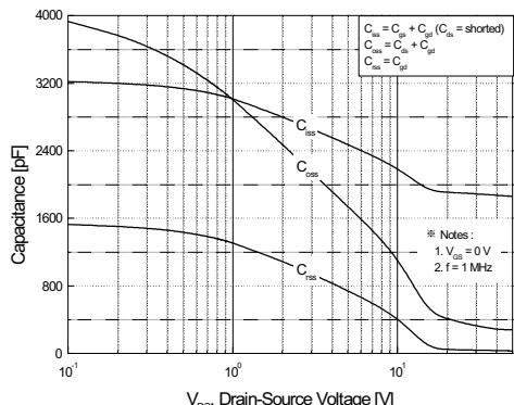
**Figure 5. Capacitance Characteristics**
