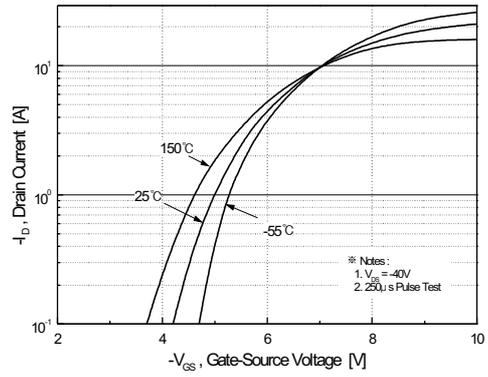
Figure 2. Transfer Characteristics
