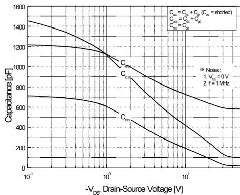
Figure 5. Capacitance Characteristics
