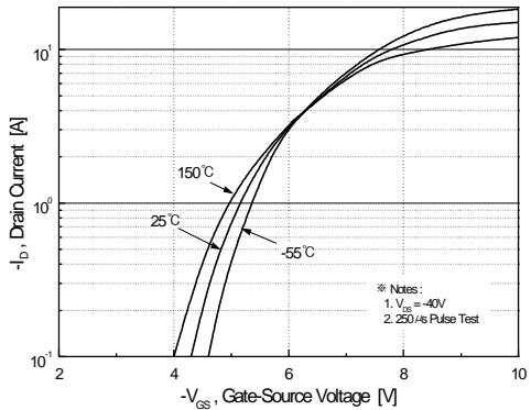
**Figure 2. Transfer Characteristics**
