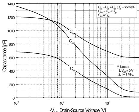
**Figure 5. Capacitance Characteristics**
