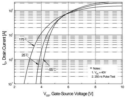
**Figure 2. Transfer Characteristics**
