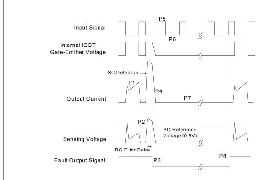
P1: Normal operation - IGBT ON and conducting current
