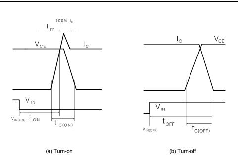
Fig. 4. Switching Time Definition
