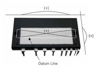
Fig. 8. Flatness Measurement Position of The Ceramic Substrate
