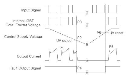
P1: Normal operation - IGBT ON and conducting current
