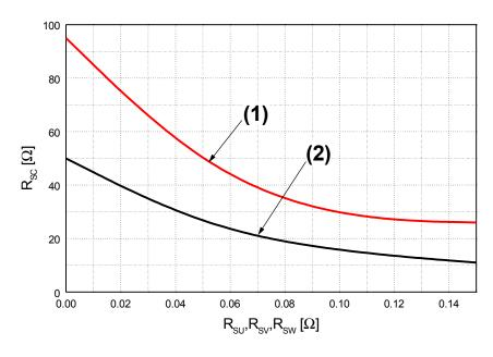
Fig. 7. R<sub>SC</sub> Variation by change of Shunt Resistors ( R<sub>SU</sub>, R<sub>SV</sub>, R<sub>SW</sub>) for Short-Circuit Protection (1) @ around 100% Rated Current Trip (I<sub>C</sub> := .10A), (2) @ around 150% Rated Current Trip (I<sub>C</sub> := .15A)
