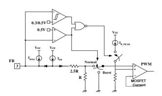
Figure 9. Circuit for Burst operation
