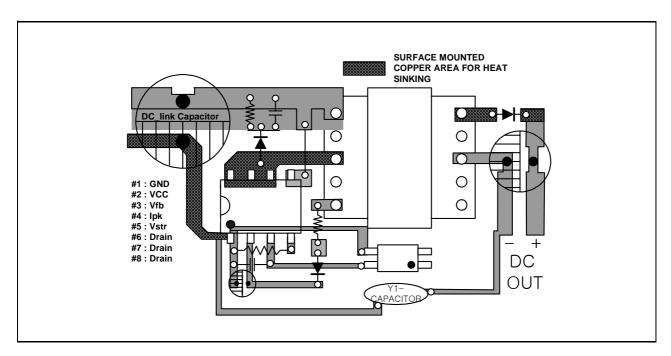
Figure 15. Layout Considerations for FSDL0165RN using 8DIP
