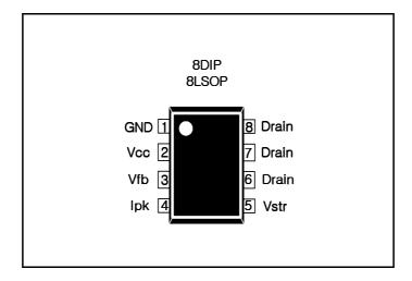
Figure 3. Pin Configuration (Top View)
