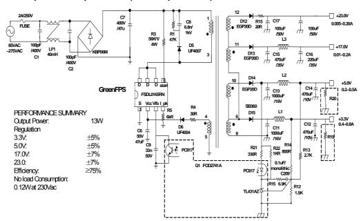
Figure 15. 13W multiple power supply using FSDL0165RN
