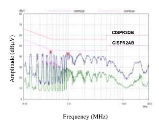
Figure 13. FSDX-series FPS<sup>TM</sup> Full Range EMI Scan (67KHz, with Frequency Modulation) with DVD Player SET
