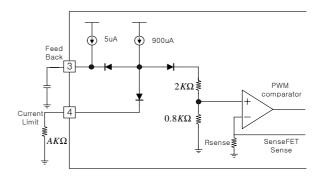
Figure 14. Peak current adjustment
