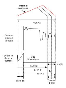
Figure 11. Frequency Modulation Waveform
