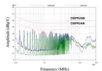
Figure 12. KA5-series FPS<sup>TM</sup> Full Range EMI scan(67KHz, no Frequency Modulation) with DVD Player SET
