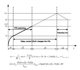
Figure 6. Over load protection
