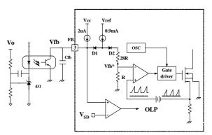
Figure 5. Pulse width modulation (PWM) circuit
