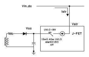
Figure 4. High voltage current source
