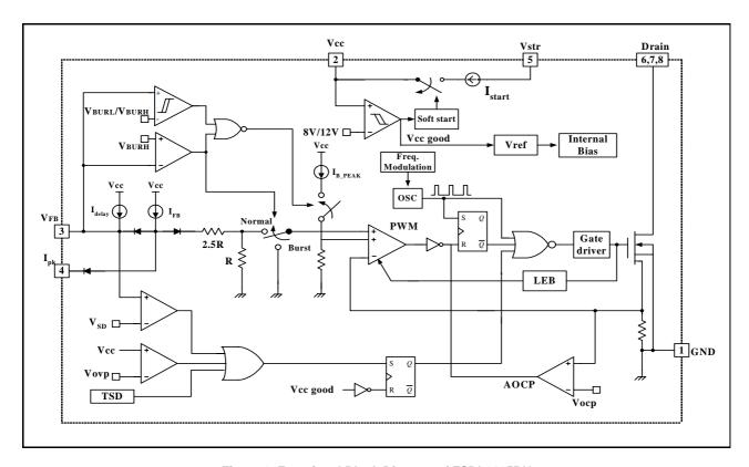
Figure 2. Functional Block Diagram of FSDL0165RN
