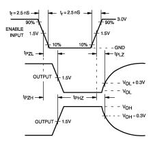
FIGURE 2. AC Waveforms
