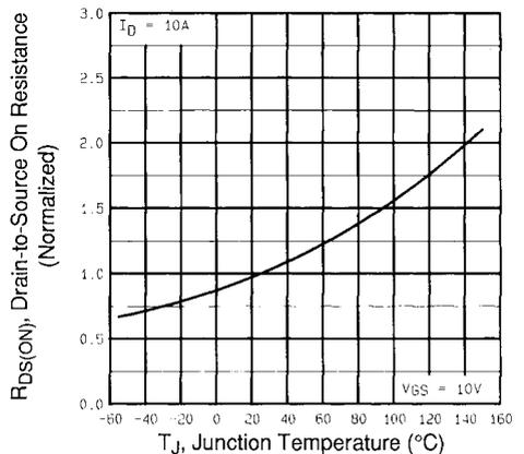
**Fig 4.** Normalized On-Resistance
