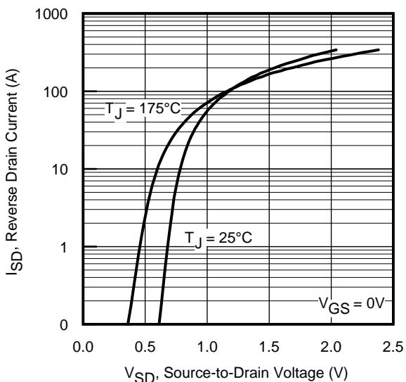
**Fig 7.** Typical Source-Drain Diode
