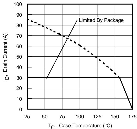
**Fig 9.** Maximum Drain Current vs.
