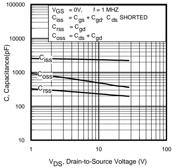
**Fig 5.** Typical Capacitance vs.
