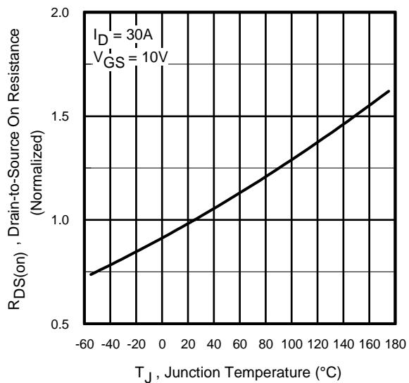
**Fig 4.** Normalized On-Resistance
