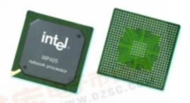
With their Development Platform, a choice of operating systems, and a broad range of development tools, the Intel IXP425 network processors provide a complete development environment for faster time-to-market. This network processor family offers the choice of multiple clock speeds at 266, 400, and 533 MHz, with both Commercial (0° to 70° C) and Extended (-40° to 85° C) temperature options.
