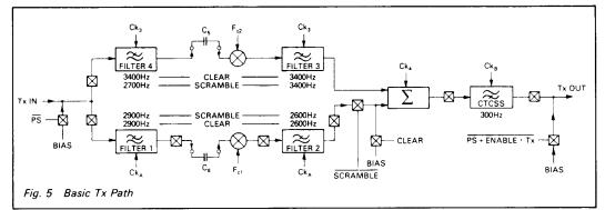
During the Transmit function the Low Pass and CTCSS filters are configured automatically as shown in Figure 5, with cut-off frequencies (-3dB) indicated.
