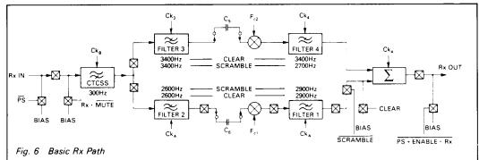
During the Receive function the Low Pass and CTCSS filters are configured automatically as shown in Figure 6
