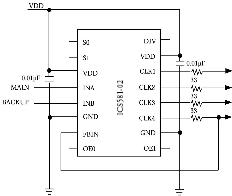
In this example, the clocks are 155 MHz and so the frequency range is address 11. Both S0 and S1 are left unconnected and so the on-chip pull-ups give the required high inputs. Similarly for OE0, OE1 and DIV. In this example, CLK4 is used as the feedback.
