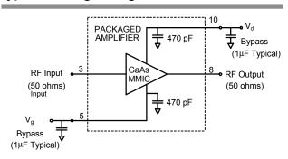
External Components Required: Bypass Capacitors: 1μ F, typical 50 Ohm microsrtip interface
