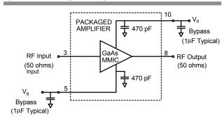
External Components Required: Bypass Capacitors:  $1\mu$  F, typical 50 Ohm microsrtip interface
