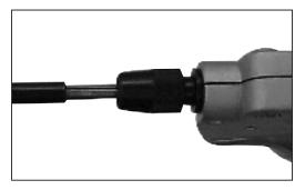
\* While squeezing the trigger, tighten the nose piece. This will insure proper orientation of the bit and sleeve and will minimize drag on the trigger.
