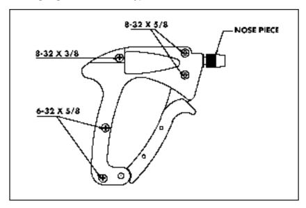
Turn the gun over and lay it down on a flat surface so the nose piece is facing left. Separate the housings and remove the collet and nose piece. Note: Use a flat head screwdriver to separate the housings.  Apply grease to the bevel, spur and face gear.
