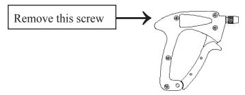
Place the G100-FL/FLA assembly on the wire wrapping gun as shown and insert the set screw and tighten. Do not over tighten.
