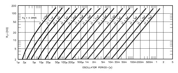
FIGURE 7. OSCILLATOR PERIOD VS.  $\rm R_T$  AND  $\rm C_T$
