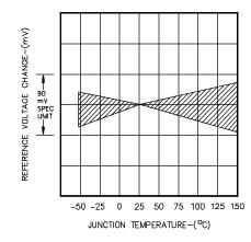
FIGURE 2. REFERENCE TEMPERATURE STABILITY
