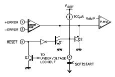
FIGURE 19. SOFT-START CIRCUIT SCHEMATIC
