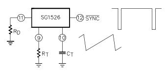
FIGURE 21 - OSCILLATOR CONNECTIONS AND WAVEFORMS
