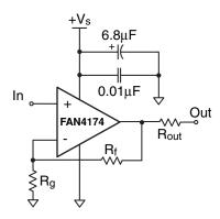
Figure 1: Typical Non-inverting Configuration
