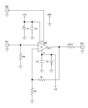
Figure 5: FAN4174 Evaluation Board Schematic
