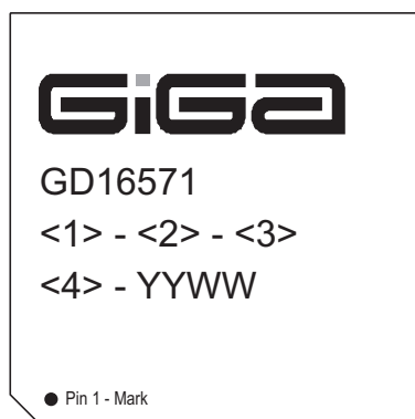
Figure 5. Device Marking, Top View.
