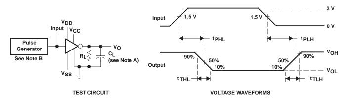
NOTES: A. C<sub>I</sub> includes probe and jig capacitance.
