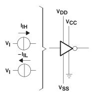
Figure 2. Driver Test Circuit for  $I_{\mbox{\scriptsize IH}}$  and  $I_{\mbox{\scriptsize IL}}$
