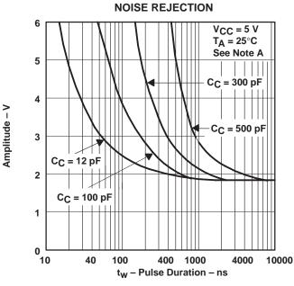
NOTE A: This figure shows the maximum amplitude of a positive-going pulse that, starting from 0 V, does not cause a change of the output level.
