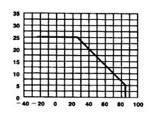
TA AMBIENT TEMPERATURE C Fig.4 MAXIMUM ALLOWABLE DC CURRENT PER SEGMENT CS. A FUNCTION OF AMBIENT TEMPERATURE.
