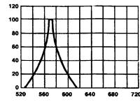
WAVELENGTH (λ)-nm Fig.2 SPECTRAL RESPONSE
