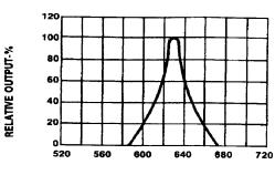
WAVELENGTH ( $\lambda$ )-nm Fig.2 SPECTRAL RESPONSE
