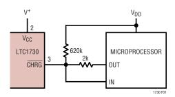
Figure 1. Interfacing with Microprocessor
